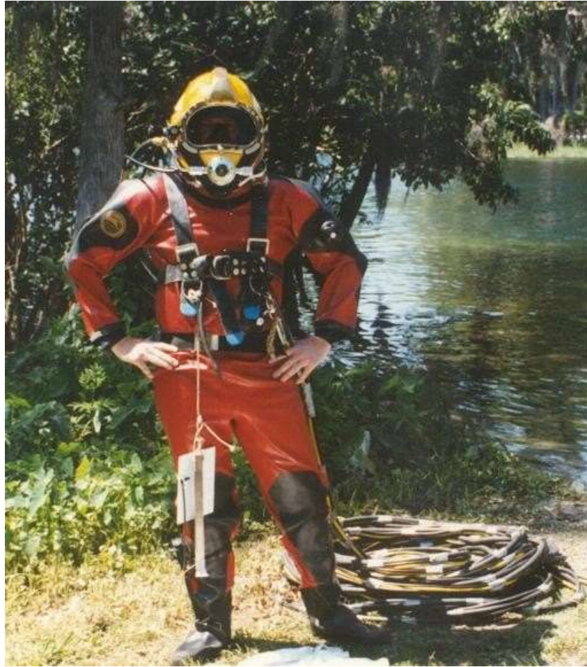
Figure 13.2.29 Surface Supplied Air Diving Equipment
